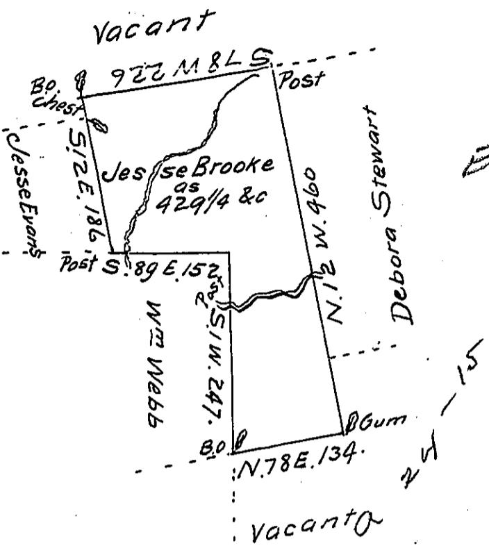
A Draft of a tract of Land called \_\_\_\_\_ situate <sup>on Beaver Creek</sup> in the County of Northumberland containing Four hundred & twenty nine acres  $\frac{1}{4}$  & 85 allow<sup>e</sup>. Surveyed for Jesse Brooke the 10<sup>th</sup> day of August <sup>1793</sup> by virtue of a warrant dated the 3<sup>d</sup> day of January 1793.
